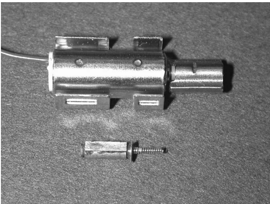
Figure 11.9 Comparison between the piezo-ultrasonic motor (bottom) and the EM motor (top), with similar power levels.
