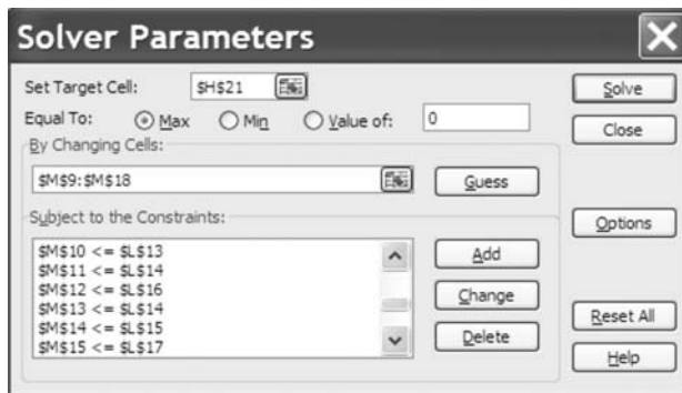
Figure 7.21 Solver Parameters dialog box setting for the PERT maximization process (backward pass).
