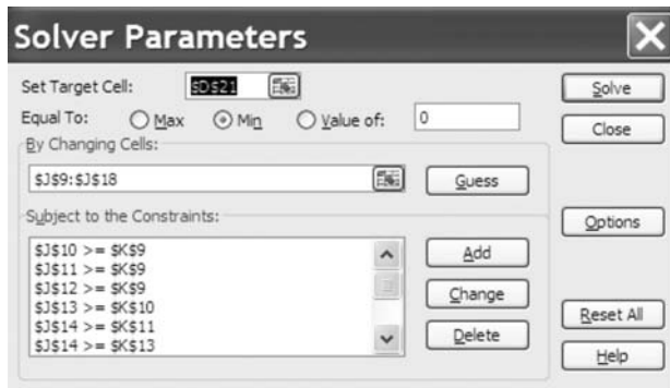
Figure 7.20 Solver Parameters dialog box setting for the PERT minimization process (forward pass).
